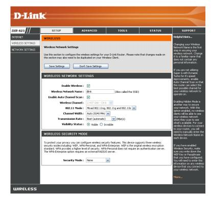
Visibility Status: Select Invisible if you do not want the SSID of your wireless network to be broadcasted by the DIR-625. If Invisible is selected, the SSID of the DIR-625 will not be seen by Site Survey utilities so your wireless clients will have to know the SSID of your DIR-625 in order to connect to it.
